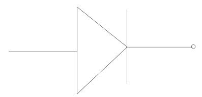
Junction diode is a solid state two terminal device which conducts with zero resistance when
