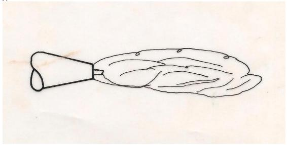
Application: It has equal volumes of oxygen and acetylene (50-50) with the inner cone well defined. It is used for welding steel, copper, aluminum, cast iron.
