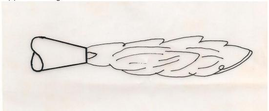
Application: It contains excess oxygen which results in oxygen rich zone beyond the cone and inner cone is sharply defined. It is used for welding brass and brass alloys.
