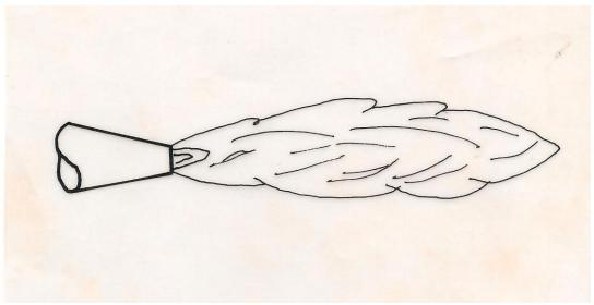
Application: It contains excess acetylene which results in carbon rich zone extending around and beyond the inner cone. It is used mainly for hard surfacing.
