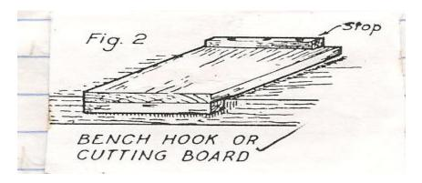
Uses: - Used to hold the job while sawing or chiseling and at the same time protecting the bench.
