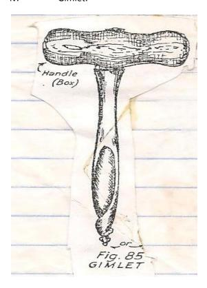
Uses: - A boring tool similar to a nail bit having a small cross handle; fitted to it for hard boring of holes for nails and screws where a brace cannot be used.
