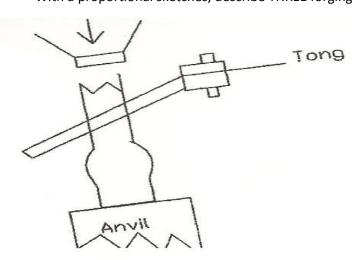
1. Upsetting is a forging operation in which the cross sectional area of the material (work piece) is increased at the expense of the length.
