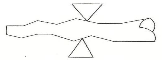
2. Drawing down is a forging operation in which the length of the material (work piece) is increased at the expense of the cross-sectional area.
