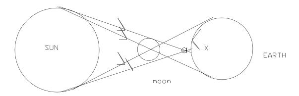
This occurs when the extreme rays at the moon's edge intersect before reaching the Earth as shown above. A ring of light is formed round the moon's shadow. The observer can be anywhere inside the region X on the Earth.
