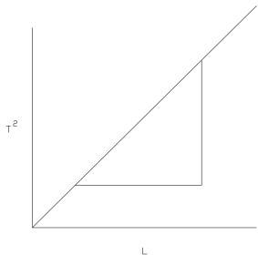
The shape of the graph  $S = (4\prod^2)$ ; from which  $g = 4\prod^2/s$ ; acceleration due to gravity at the place the experiment was performed.
