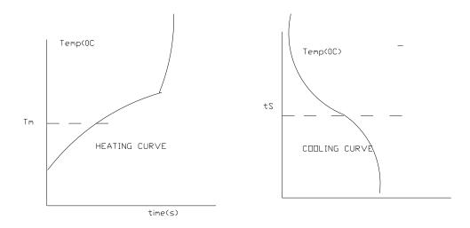
Precautions:- (1) Thermometer must always be in the midst of the Nephthalene. (2) Nephthalene must be of the highest purity (3) prevent parallax error in reading thermometer.
