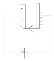
An Insulator called a dielectric may be placed in the space between the plates in close contact with them.
