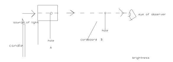
A small hole is punched in each of the cardboards A and b. They are placed in a straight line together with a light source. An observer is situated on the other side B. it will be found that the observer can only see light if the cardboards are well aligned. Light will pass through both holes.
